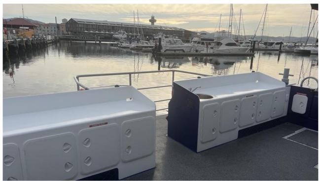
• Below: image of bow area on boat. Handrails around 70 cm wide external walkway, or 70 cm wide door from cabin.
